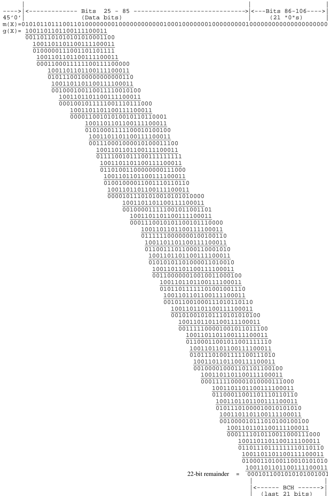
Figure B1: Sample 21-Bit BCH Error-Correcting Code Calculation
